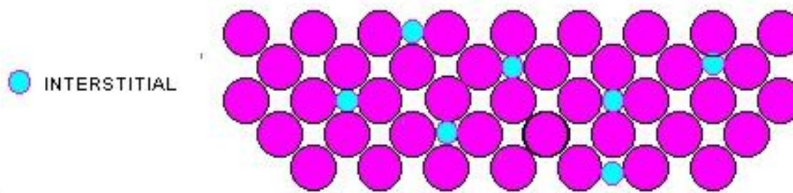
SOLUTE ATOMS MUST BE SMALL IN SIZE < .59 DIAMETER OF SOLVENT ATOMS
