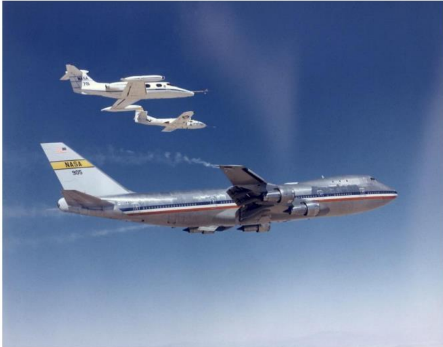
Dryden Flight Research Center ECN-4243 Photographed 1974 747 wake vortex research with smoke generators. A Learjet and T-37 Cessna fly through the wake. NASA photo
