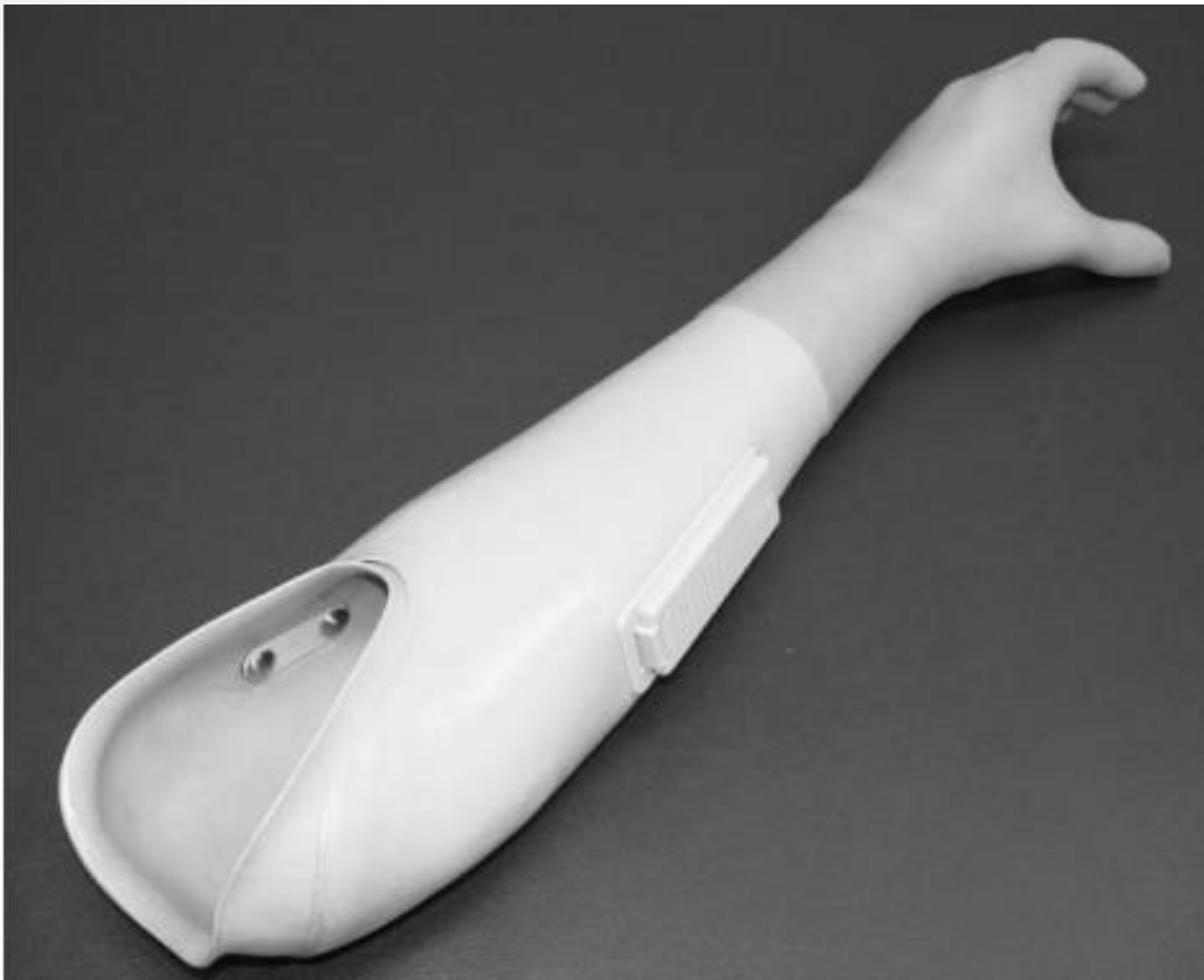
Myoelectric transradial prosthesis. The electrode embedded within the socket detects surface electromyogram (EMG) activity
