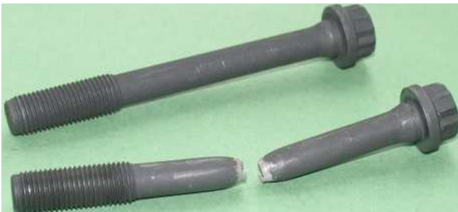
Figure 3.9.1 Failure in tension (necking)
